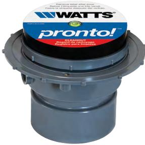
Watts Pronto!® CO-1190-PR-60 PVC floor cleanout with anchor flange, post-pour adjustable round stainless steel strainer with integrated bubble level, leveling shims, and PVC socket outlet (standard).
