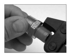
2. Rotate the fitting 180° and completely close the tool. Remove ring.
