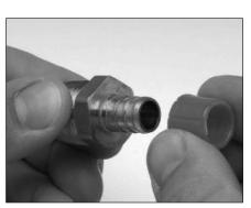
**Important:** After removal of crimp ring, carefully inspect the barbs on the fitting. If barbs are scratched or deformed, discard the fitting, and do not reuse. Leaks may occur on damaged fittings that are reused.
