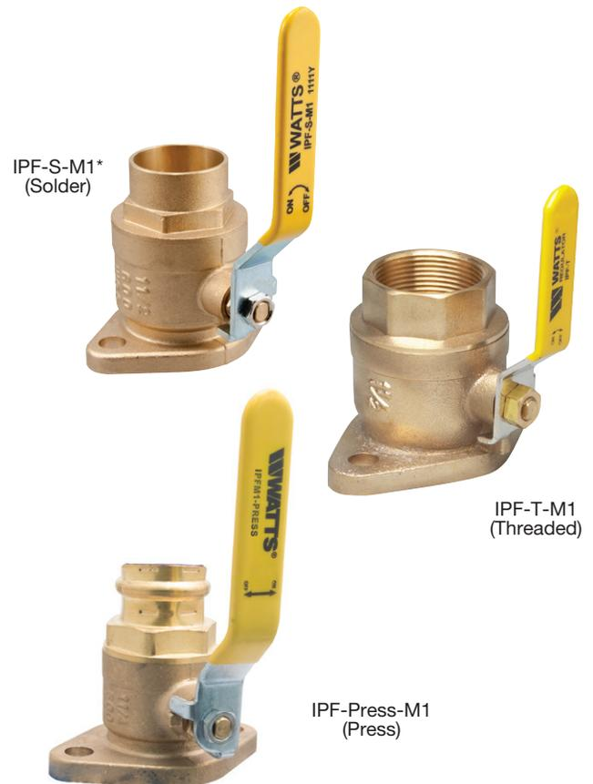
\*This valve is designed to be soft soldered into lines without disassembly, using a low temperature solder to 420°F (216°C). Higher temperature solders may damage the seat material.
