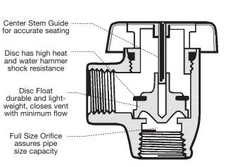
Since atmospheric type vacuum breakers are subject to normal maintenance and replacement, they should be located where emergency water spillage will create no problem and where they can be accessible for inspection or servicing.
