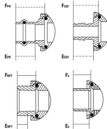
VALVES MAY BE ORDERED WITH 0, 1, OR 2 UNION CONNECTIONS USING ANY COMBINATION OF NPT, SOLDER, CEF (F1960), OR PRESS CONNECTIONS REQUIRED
