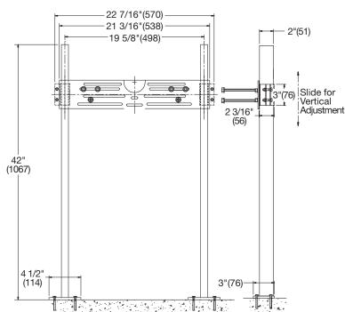
Note: Anchor legs to concrete floor with minimum 1/2"(13) anchor bolts (by others).
