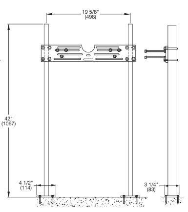
Note: Anchor legs to concrete floor with minimum 1/2"(13) anchor bolts (by others).
