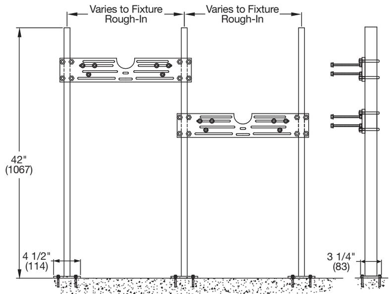
Note: Anchor legs to concrete floor with minimum 1/2"(13) anchor bolts (by others).
