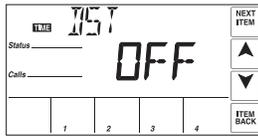
Turn daylight savings time ON if an automatic time change is required.
