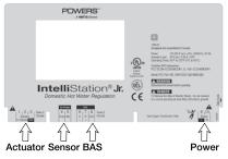
11. Reconnect the sensor, actuator, BAS (if used) and power wires.
