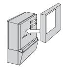
14. Position the front cover onto the unit, then snap it in place.
