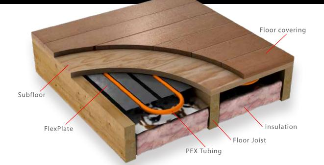
FlexPlate is a revolutionary new type of under floor heating plate. The primary material in the plate is a specially processed natural graphite, giving FlexPlate 50% higher thermal conductivity than aluminum. Extensive performance testing indicates FlexPlate will outperform the extruded aluminum plates.
