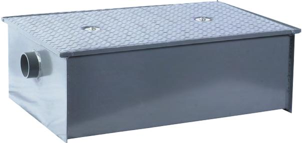
Watts WD-L Series PDI Certified recessed or floor mounted epoxy coated steel low-rough-in grease interceptor with gasketed skid-proof cover secured with hex head center bolts, removable baffle assembly, deep seal trap with cleanout and air relief bypass, external vented flow control fitting, and no hub (standard) connections.
