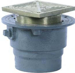
Watts CO-200-SX epoxy coated cast iron floor cleanout with 5" x 5"(127x127) square adjustable gasketed heavy duty nickel bronze top, removable gas tight gasketed brass cleanout plug, and no hub (standard) outlet.
