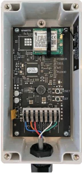
Control Cable, 6 conductors, 22 AWG, PVC conductor insulation material for the Cellular Gateway
