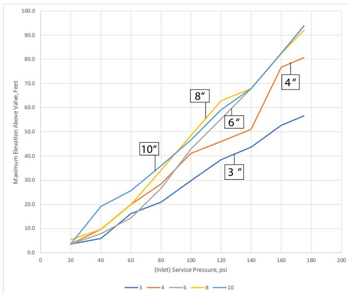
Graph is based upon 1/2" (15 mm) pilot sprinklers installed on 1/2" (15 mm) schedule 40 galvanized release system piping and a 500 ft. maximum pilot line length.
