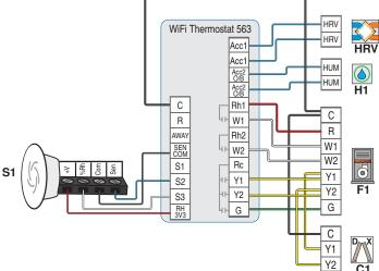
The WiFi Thermostat 563 operates a first stage radiant floor and a second stage fan coil for heating, and two-stage air conditioner for cooling and dehumidification, and a humidifier.
