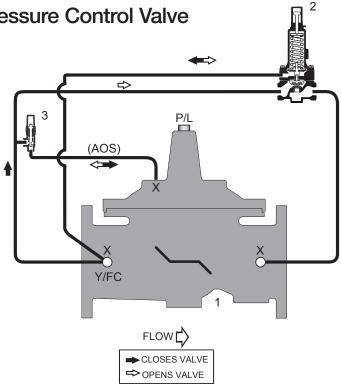
toward a closed position, sustaining pressure in the upstream zone. The valve will close, if necessary, until upstream pressure is above the pilot setting. The valve should be specified to include the optional opening speed control and position indicator when used for Pressure Sustaining applications.
