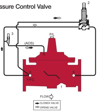
toward a closed position, sustaining pressure in the upstream zone. The valve will close, if necessary, until upstream pressure is above the pilot setting. The valve should be specified to include the optional opening speed control and position indicator when used for Pressure Sustaining applications.
