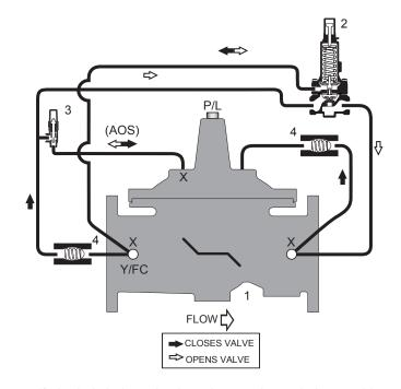
specified to include the optional opening speed control when used for Backpressure applications.
