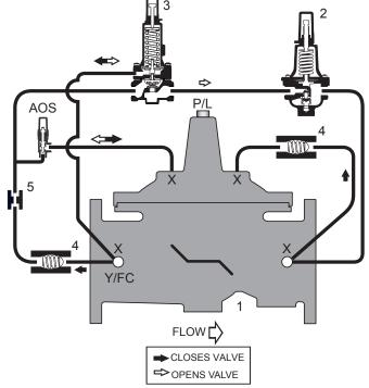
If downstream pressure becomes greater than upstream pressure, downstream pressure is admitted to the main valve cover chamber, closing the valve and preventing reversal of flow. Normal backpressure or sustaining operation resumes when upstream pressure exceeds downstream pressure.
