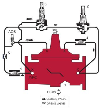
If downstream pressure becomes greater than upstream pressure, downstream pressure is admitted to the main valve cover chamber, closing the valve and preventing reversal of flow. Normal backpressure or sustaining operation resumes when upstream pressure exceeds downstream pressure.
