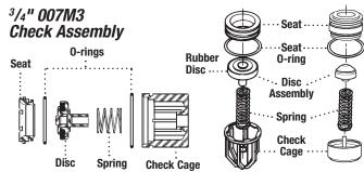
Rubber seat disc can be replaced. However, disc holder and disc retainer are permanently bonded to prevent failure.
