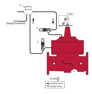
trolled by the adjustable opening speed control, which restricts the speed at which fluid and pressure evacuate the cover chamber. When the valve reaches the full open position, the limit switch is actuated, turning the pump off.
