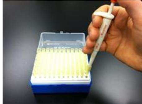
2. Depress the operating button on the top to the first stop (see photo at left). **DO NOT depress all the way to body.**
