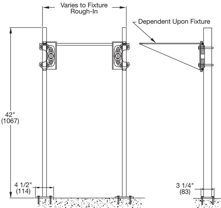
Note: Anchor legs to concrete floor with minimum 1/2"(13) anchor bolts (by others).
