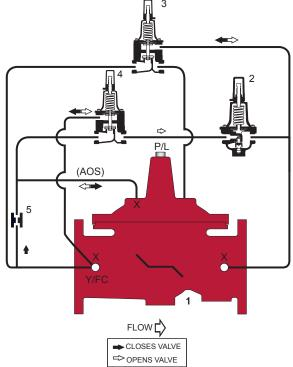
ing the valve to modulate toward a closed position, raising upstream pressure. Normal pressure reducing operation resumes when upstream pressure is above the sustaining pilot setpoint, and downstream pressure is below the reducing pilot setpoint.
