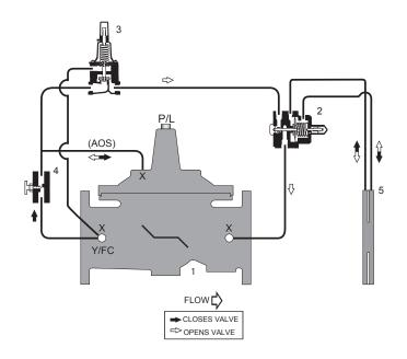
The normally closed sustaining pilot remains open when upstream pressure is above the adjustable setpoint, and modulates toward a closed position if upstream pressure falls below the setpoint. As the sustaining pilot closes, fluid is directed into the main valve cover chamber, allowing the valve to modulate toward a closed position, raising upstream pressure. Normal flow control operation resumes when upstream pressure is above the sustaining pilot setpoint.
