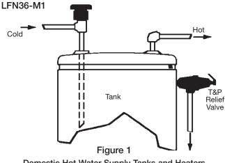
Domestic Hot Water Supply Tanks and Heaters with Top Supply
