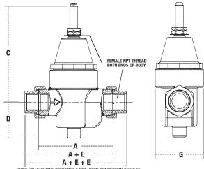
ABOVE VALVE SHOWN WITH SINGLE NPT UNION CONNECTION ON INLET VALVES MAY BE ORDERED WITH 0, 1, OR 2 UNION CONNECTIONS USING ANY COMBINATION OF NPT, SOLDER, PEX OR CPVC CONNECTIONS REQUIRED
