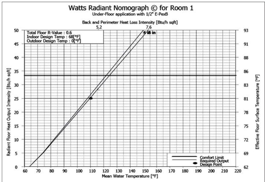
PEX with Plates Nomograph showing a supply temperature of 120° with a BTU load of 25 BTU/sqft and floor surface temperature of 81°F.
