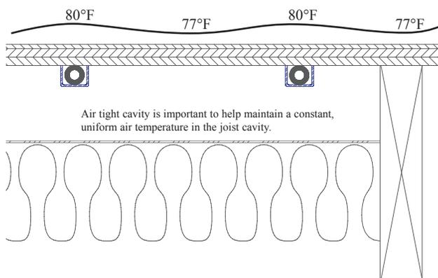
from the subfloor. This separation decreases the tubing's ability to transfer energy to the subfloor, and reduces its overall heating ability.
