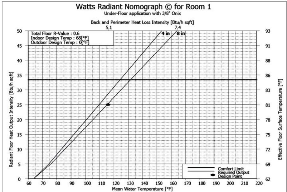
Onix Staple-Up Nomograph showing a supply temperature of 125° with a BTU load of 25 BTU/sqft and floor surface temperature of 81°F.
