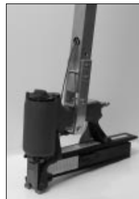
Extension Arm on staple gun fitted with Onix Guide plate.
