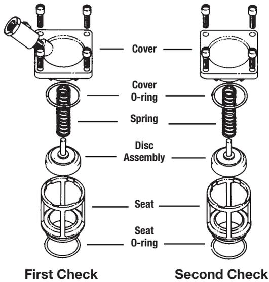
1. Remove the four screws holding the first check valve cover.
