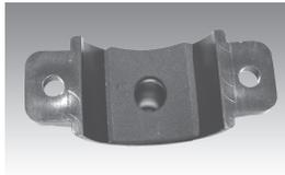
**Step C** – The drain saddle must be installed at least 1½" above the nut of the P-Trap elbow or cross bar from the garbage disposal to insure proper drainage. Using the ¼" drill bit, drill into the drain pipe at best available location as specified above, for drain saddle installation. Take extreme caution to only drill through one side of the drain pipe.
