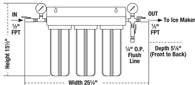
**Note:** Allow 3" of clearance at bottom of system for removal of filter bowls for filter cartridge replacement
