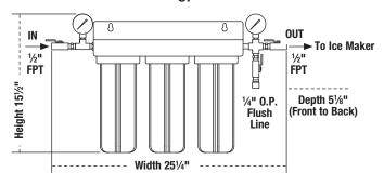
Note: Allow 3" of clearance at bottom of system for removal of filter bowls for filter cartridge replacement
