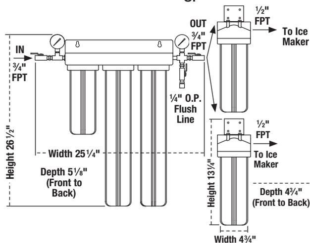
**Note:** Allow 3" of clearance at bottom of system for removal of filter bowls for filter cartridge replacement
