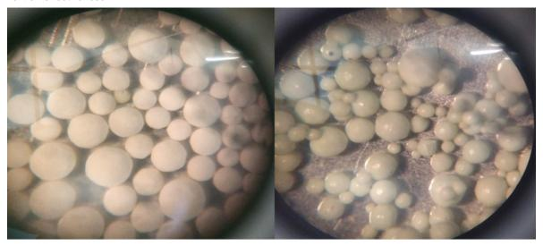
Figure 8. MAC media comparison - new (left) vs. fouled (right)
