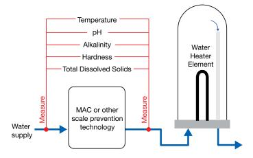
Figure 1. Scale prevention testing schematic
