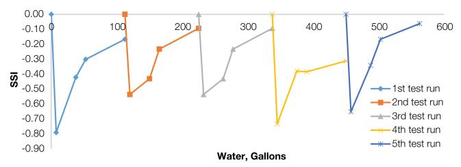
Figure 5. SSI of new MAC media testing in TX
