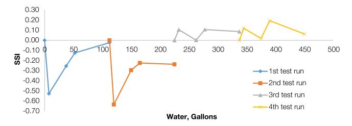
Figure 7. SSI of MAC media testing with feed water of residual copper
