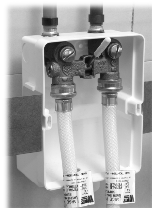
Single-lever Water Off Washing Machine Control Center with 1/2" (15mm) CrimpRing™ fittings and flexible PVC supply lines.
