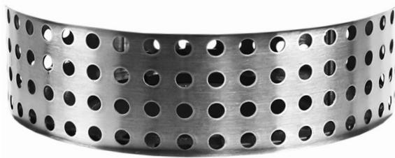
The **-W Adjustable Internal Water Dam** option is a pipe inserted in the middle of the roof drain that holds water back until it reaches a certain height on the roof.
