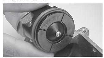
3. When installing the check modules, make sure the check assembly with the heavy duty spring is inserted in the inlet bore of the body (first check position). Position the first check assembly so that one (1) of the four (4) flow path windows is face-down toward the relief valve. The check assembly with the weaker spring must be installed in the outlet bore of the body (second check position).
