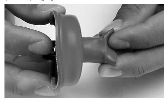
6. Apply a thin coating of the supplied lubricant to both sides of the second slip ring (Item 18.1) and place it over the top of the small diaphragm, making sure the outer diaphragm (Item 16) is not folded or creased under the slip ring. Push the slip ring down flat until the adhesion from the grease holds the small diaphragm in place. This should roll the diaphragm as shown. Thread the brass cylinder (Item 18) into the relief valve cover and hand tighten.
