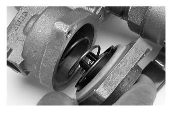
8. After reassembly, with all test cocks closed, slowly open the inlet ball valve and bleed air from the unit by opening and closing test cock No. 2, No. 3, then No. 4.
