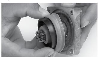
4. Apply a thin coating of the supplied lubricant to both sides of the new seat gasket ring (Item 12.1), and slide it on the short end of the new seat ring (Item 12). Slide the short end of the new seat ring into the hole of the relief valve body. (The adhesion from the lubricant holds the seat ring in place during the rest of the assembly process.)
