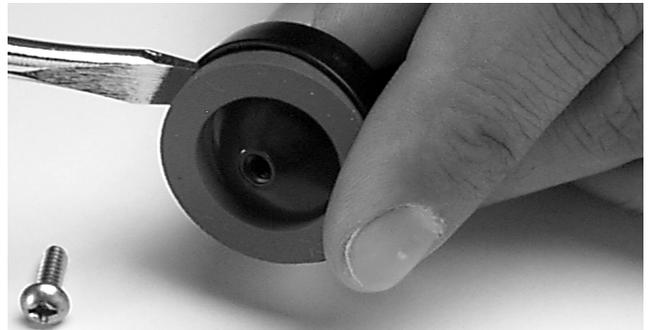
3. Reassemble the check module by reversing the preceding steps. When reassembling the check module, insert the poppet stem into the guide hole and keep fingers clear of the slots in the module.
