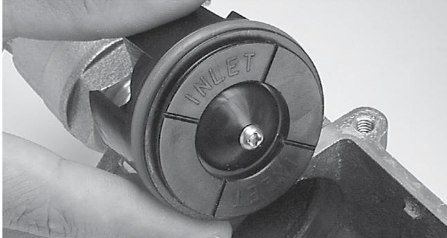
3. When installing the check modules, make sure the check assembly with the heavy duty spring is inserted in the inlet bore of the body (first check position). Position the first check assembly so that one (1) of the four (4) flow path windows is face-down toward the relief valve. The check assembly with the weaker spring must be installed in the outlet bore of the body (second check position).
