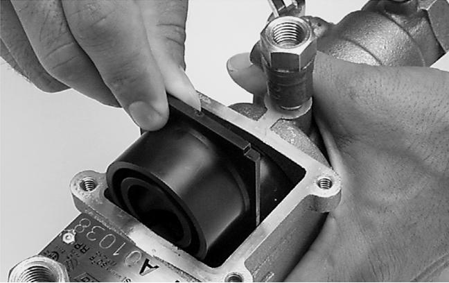
4. Remove the inlet check assembly by pulling it in the direction of flow from the body bore until it is completely exposed, then lift it out of the body.
