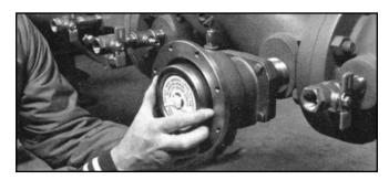
Replace the cover, tighten the cover bolts, and reconnect the sensing tubing. Return to service and test the assembly to ensure proper operation.
