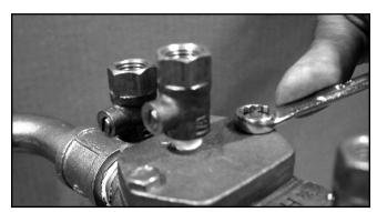
Carefully place the relief valve body over the bushing and tighten the two cap screws to retain the relief valve body to the main valve body. New cap screw sealing washers should be installed to avoid leakage.
