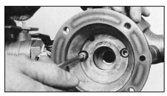
4. Lubricate the O-rings and main stem using FDA Approved lubricant. Place the main stem and spring into the guide and replace the flathead screw located at the center button.
