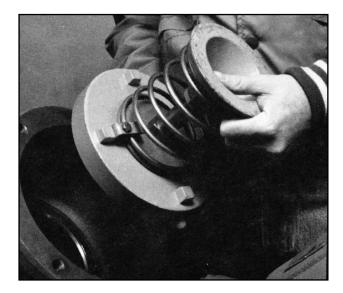
Unthread the retaining nut from stem and remove the disc washer and seat disc.
