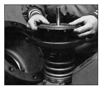
2. Inspect seat disc for wear or damage. Replace with the new seat disc or turn used disc over if a new disc is unavailable.
