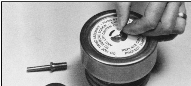
5. To reassemble, position the bead on the inner diaphragm into the groove of the upper guide. Place the slip ring over the diaphragm. Lubricate the retainer threads using an FDA Approved lubricant and thread the retainer onto the upper guide. Tighten to 60 inch-lb of torque.
