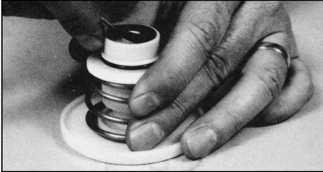
5. To remove spring and/or main stem from the guide, keep the unit compressed and remove the screw (item 18) located in the center of the button. Push the main stem through the guide and remove the O-ring from the main stem. Inspect and clean or replace the O-ring and seat disc as required. Clean all parts thoroughly with clean water before reassembly.
