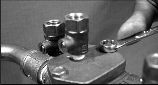
3. Carefully place the relief valve body over the bushing and tighten the two cap screws to retain the relief valve body to the main valve body. New cap screw sealing washers should be installed to avoid leakage.
