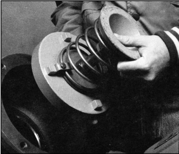
1. Unthread the retaining nut from stem and remove the disc washer and seat disc.
