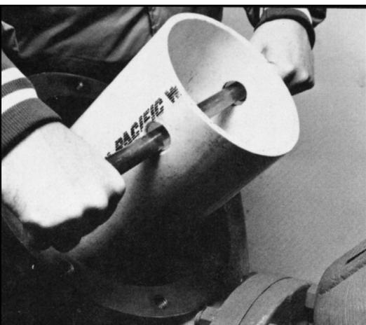
1. Remove the check valve as described in the preceding procedure.
