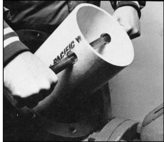
2. Remove the bushing and bushing nut (items 2A and 2B).
