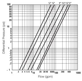
Flow curves show flows (gpm) and pressure drop (psig) through Series A777SI using 20 mesh screen.
