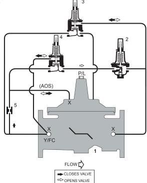
ing the valve to modulate toward a closed position, raising upstream pressure. Normal pressure reducing operation resumes when upstream pressure is above the sustaining pilot setpoint, and downstream pressure is below the reducing pilot setpoint.
