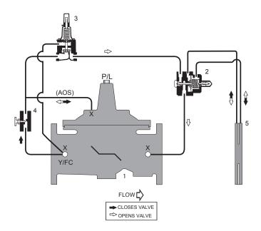
The normally closed sustaining pilot remains open when upstream pressure is above the adjustable setpoint, and modulates toward a closed position if upstream pressure falls below the setpoint. As the sustaining pilot closes, fluid is directed into the main valve cover chamber, allowing the valve to modulate toward a closed position, raising upstream pressure. Normal flow control operation resumes when upstream pressure is above the sustaining pilot setpoint.
