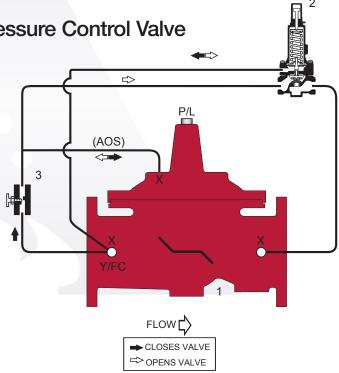
The valve will close, if necessary, until upstream pressure is above the pilot setting. The valve should be specified to include the optional opening speed control and position indicator when used for Pressure Sustaining applications.
