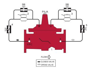
The valve is constructed with two "normally closed" solenoids allowing the valve to "hold last position" upon power failure. The valve may also be configured to open fully or close drip tight upon power failure if desired by using one "normally closed" and one "normally open" solenoids.
