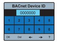
To adjust the ID depress the **Del** key 7 times and enter an ID appropriate for the remainder of the BAS system and press **OK**. Similarly, enter an appropriate "BACnet Port." To change "Register Foreign Dev" to "ON" scroll down to "Register Foreign Dev" using the **Up** and **Down** icons and select **Enter**. The "Register Foreign Dev" setting adjustment screen is shown in the "OFF" state below.
