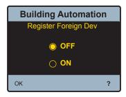
To toggle from "OFF" to "ON" press on the indicating that this state is what is selected. Press OK to save this setting and return to the "Building Automation" menu shown below with "Register Foreign Dev" set to "ON". Note the additional setting available with the "Register Foreign Dev" set to "ON."
