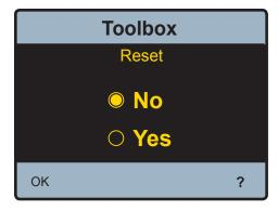
Press the **OYes** and then **OK** and the control will reset and begin a start up sequence.
