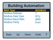
The "Modbus Address" setting adjustment screen is shown below.
