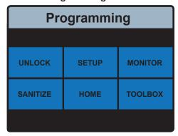
On the "Programming" Menu the UNLOCK and HOME icons are the only active icons until the control is unlocked. See "Unlock the System" in the "Set up and Programming" section of this Manual.
