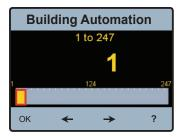
To adjust the "Modbus Address" either press anywhere on the slider bar use the arrow keys and then select OK) save the setting and return to the "Building Automation" menu. The "ModBus Baud Rate" and "Modbus Parity" are adjusted in a similar fashion.
