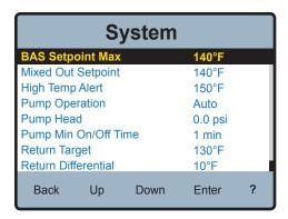
2. Selecting and Setting Outlet Water Temperature Set-point:
