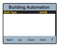
The default "BAS Type" is "NONE" as shown above. To change this setting press the "Enter" icon and the "BAS Type" adjustment screen will appear (as shown below).
