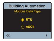
To toggle from "RTU" to "ASCII" press on the icon next to the "ASCII" setting to change the indicating that this state is what is selected. Press indicating that this state is what is selected. Press indicating Automation is menu.
