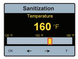
Next, select the run time in minutes by first highlighting the TIME function on the Sanitization menu and touching Enter.
