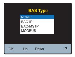
Depress the UP and Down icons to scroll through the BAS types and depress the OK icon to configure the control to the highlighted type and return to the "Building Automation" menu. Note: depending on the "BAS Type" selected, various user configurable items will now appear within the "Building Automation" menu. A table of the user definable items is shown on the next page.
