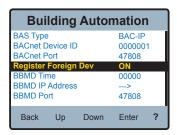
The "BBMD Time" and "BBMD Port" are adjusted similarly to the "BACnet Device ID." The "BBMD IP Address" adjustment screen is shown below.
