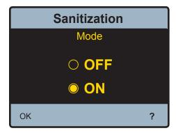
The Sanitization Mode is now fully functional. Note: The HOME screen will indicate you are Sanitizing the water delivery system and indicate Mixed Outlet Temperature.
