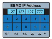
Use the Tab icon to move between the four groups of three numbers, use the to move around in each group of 3 numbers, and use the Del to delete the numbers entered in the field to allow entering a new number.
