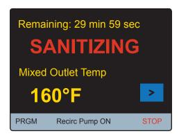
After Sanitization Mode has completed (user selected run time has elapsed), the IntelliStation will go into a Cool Down Mode to return to the Mixed Outlet temperature prior to sanitizing.
