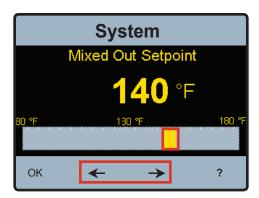
4. Select and set the safe, appropriate and desired outlet water temperature for your users, application and facility by using the slider icon or by touching the right or left arrows until the selected temperature is displayed.
