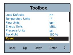
From within the "Toolbox" menu use the Down icon to highlight "Reset" as shown above then press Enter. This will access the "Reset" menu shown below.
