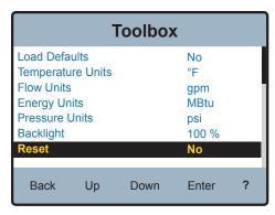
From within the "Toolbox" menu use the **Down** icon to highlight "Reset" as shown above then press **Enter**. This will access the "Reset" menu shown below.
