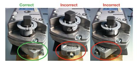
2. To adjust the armature position, depress the actuator manual override button (see below) and turn the armature to the "Correct" position shown above.
