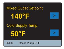
Reset the control by opening and closing the circuit breaker switch and wait 60 seconds to resume normal operation.
