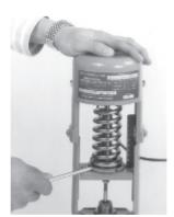
5. Adjusting Set Point © 2019 Watts
