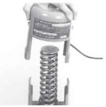
7. Remove Housing and Thermal System
